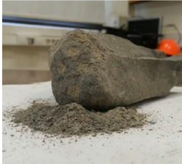
Figure 5. Self-disintegrating slag sample.
