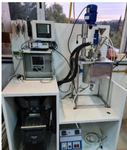
Figure 8. Lab-Pilot setup at NTUA used for investigating the fundamentals and boundaries of the precipitation process.
